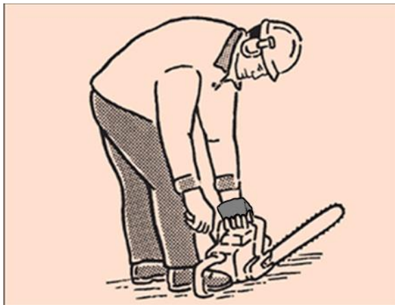
Fig 19: Cold starting method.
