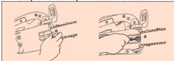
Fig 31: Adjusting the tension so the straps and cutters solidly contact the bar rail
